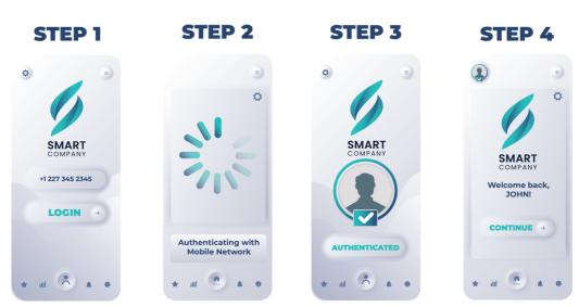
**Step Three** - The device identity is authenticated and the result is passed back to TMT Analysis out-of-band by the mobile network operator so that it cannot be intercepted/copied.
